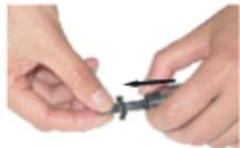
Push the cover backwards to release the mandrel. Release the mandrel by turning it counter-clockwise.
