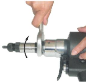
When a smaller size rivet nut is used such as M3 or M4, the stroke must be adjusted to prevent damaging the mandrel and inside thread of rivet nut.
