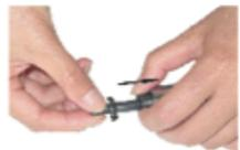
Push the cover backwards and install the replacement mandrel turning clockwise until it stops. Release the cover in install the matching nose piece.
