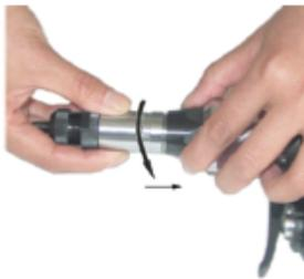
2. Turn the locknut anti-clockwise and turn the outer sleeve clockwise to shorten the stroke. Then tighten the locknut.
