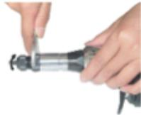
Unlock the locknut and nosepiece and remove.
